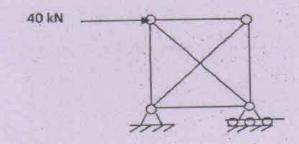
The peripheral members of truss are of length 3 mts each.
