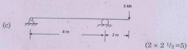
4. (a) Solve the beam in Prob 3(a) for slope and deflection at free end using moment area method. (3 + 3)
