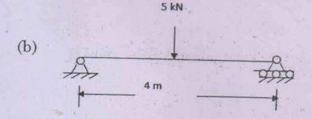
Solve the above mentioned beam for slope and deflection under the midspan load using ouble integration method. (3+3)
