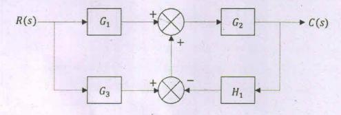
(c) Find the gain of the following signal flow graph using Mason's Gain formula. (3)
