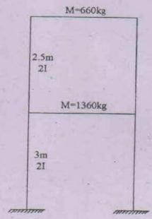
9. (a) One of the plane frame of a four storeyed RC building is shown in the figure. The building is symmetric and regular. It is situated in Guwahati. Calculate the Base Shear of the building for the given specifications.
