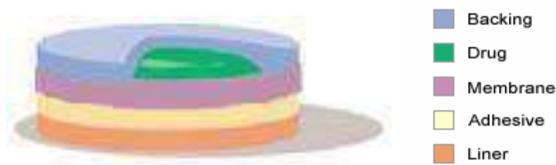
Figure 1.6: Drug reservoir in adhesive
