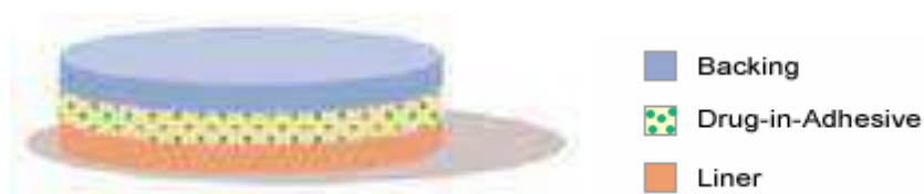
Figure 1.3: Single layer drug in adhesive
