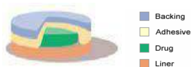
Figure 1.5: Drug matrix in adhesive
