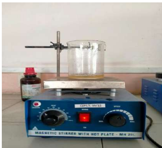
Figure 3: After being sieved by sieve no. 60 was dissolved in 90%, ethanol at 25°C, on a hot magnetic stirrer at 50 RPM.
