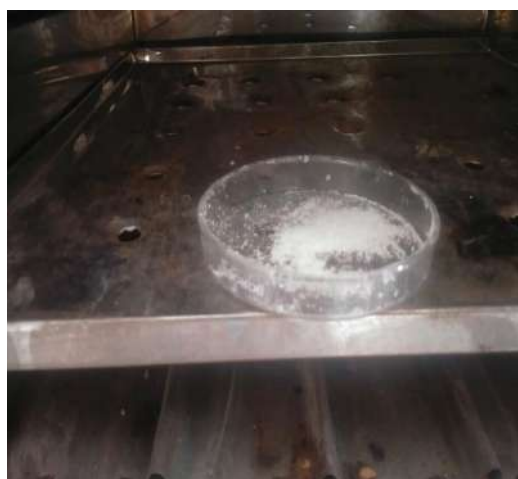
Figure 5: Then the remaining solvent was evaporated in hot air oven to make it drier & powder like, so it can be incorporated in tablets.
