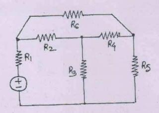
(b) Find  $I_1$  and  $I_2$  of the network using Nodal analysis. (7)
