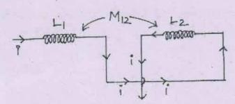
(c) The number of turns in two coupled coils are 500 and 1500 respectively. When a current of 5A flows in coil 1, the total flux in the coil is 0.6 mWb and the flux linking the 2 nd coil is 0.3 mWb? Find  $L_1, L_2$ , M and K. (5)
